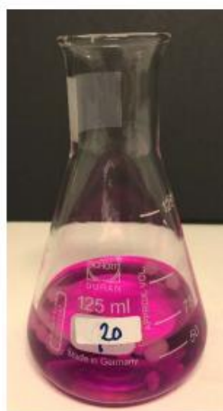
Figure 3. Chitosan beads soaking in potassium permanganate solution
